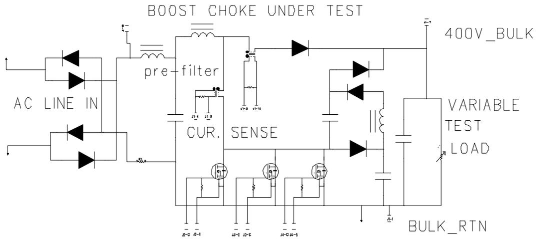
Figure 2. Continuous Conduction Mode PFC Test circuit
