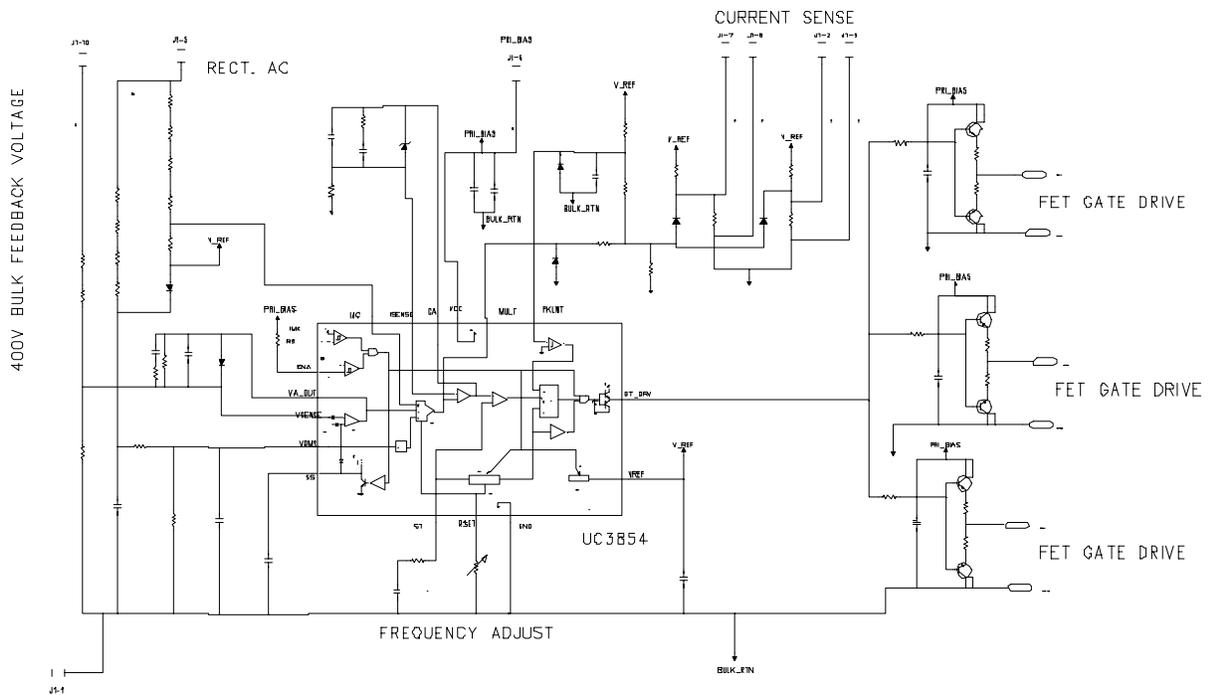
Fig. 3. Continuous Conduction Mode PFC Control Circuit
