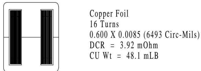
Figure 4. Comparison of winding methods via a normalized one inch by one inch winding cross section
